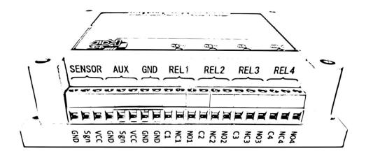
SENSOR GND OV Supply connection output for flow sensor (conect to BLACK cable)
